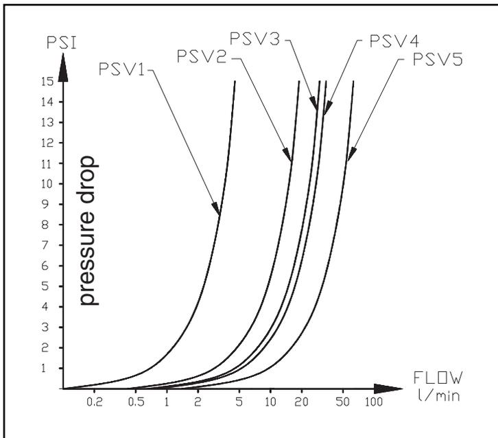
PSV Proportionating Solenoid Valves are uniquely designed to respond to variable power inputs (0-30 VDC) to regulate flow of liquids and/or gases proportionately. For added safety PSV valves are normally closed (NC) when de-energized.
