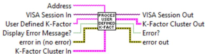
Applies "User Defined K-Factor" to currently selected Gas Table. If successful returns K-Factor Index, floating-point number with K-Factor value in the K-Factor cluster. K-Factor does not work with %FS engineering unit. Valid User Defined K-Factor Values are from 0.1 to 1000. To apply currently selected User Defined K-Factor Value leave "User Defined K-Factor" terminal empty.
