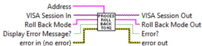
Sets/Reads currently selected "Roll Back to N2 Mode" parameter. When "Roll Back to N2 Mode" terminal is empty this Sub-VI performs "Read" function. Valid values for "Roll Back to N2 Mode" parameter are "E" or "D" strings.
