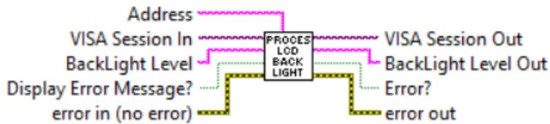
Sets/Reads LCD Back Light level parameter. Valid values for "Back Light Level" terminal are from 0 to 100% When setting new Back Light level the instrument response is in counts [0 to 4095]. When reading current Back Light level (*BackLight Level* terminal is empty) the instrument response is in % [0 to 100].
