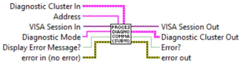
Enable / Disable LCD Diagnostic messages (only for LCD option) when "Diagnostic Mode" terminal is set to "E" or "D". When "Diagnostic Mode" terminal is empty this Sub-V reads the bitwise Diagnostic events code, Status LED state and LCD diagnostic mode (enabled/disabled).
