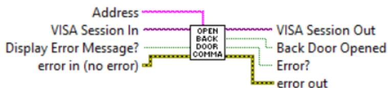
Reads Back Door status for accessing instrument's diagnostic SRAM registers. If Back Door is opened returns "TRUE" value on the "Back Door Opened" terminal. When XFM "Back Door" is opened user can use "READ" and "WRITE" ASCII command to read and write instrument's SRAM registers to troubleshoot instrument behavior.
