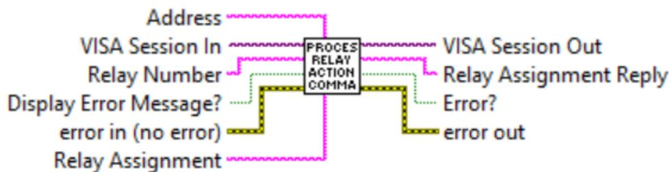
Reads and writes instrument's Relays assignment parameter. Refer to XFM ASCII commands set (Paragraph 8.3 in the XFM operating manual) to determine valid values for "Relay Number" and "Relay Assignment" input terminals.
