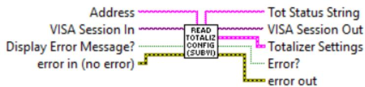
Queries instrument's Totalizer parameters, parses data frame received from the instrument and populates data in to the Totalizer Settings cluster. "Totalizer Settings" cluster represents actual Totalizer parameters it was initialized with. This sub-VI can be run at the beginning of a program outside the main loop, and should be re-run every time the instrument address is changed (for RS-485 interface).
