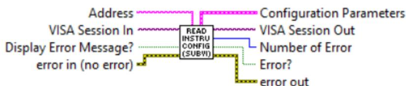
Reads instrument configuration parameters in to the "Configuration Parameters" cluster. This sub-VI can be run at the beginning of a program outside the main loop, and should be re-run every time the instrument address is changed (for RS-485 interface).
