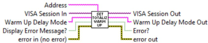
Sets instrument's Totalizer Warm Up Delay Mode:
