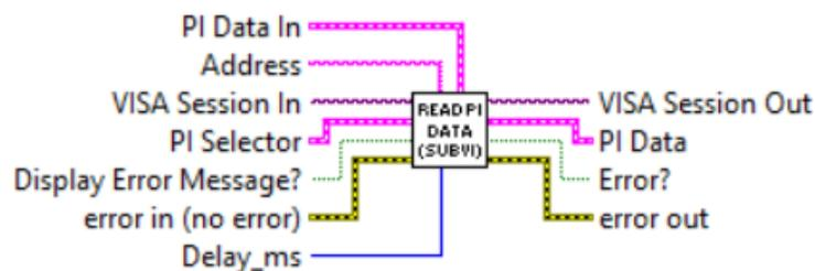
Reads the instrument's Process Information parameters: Mass Flow Rate, Totalizer reading and Flow Alarm status and composes the cluster of string representing following parameters: Mass Flow Rate (MEU), Totalizer value (MEU), Flow Alarm Status [N,H,L] and Diagnostic Register value.
