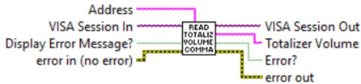
Reads current Totalizer volume in currently selected (not time based) mass flow units of measure.
