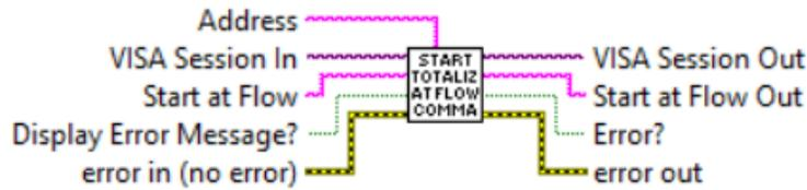
Sets Totalizer "Start At Flow" parameter. Wire floating point string with values between 0 and 100%FS to "Start at Flow" input terminal to select desired Totalizer "Start At Flow" parameter. Refer to XFM ASCII commands set (Paragraph 8.3 in the XFM operating manual) to determine valid values for "Start @ Flow" input terminal.
