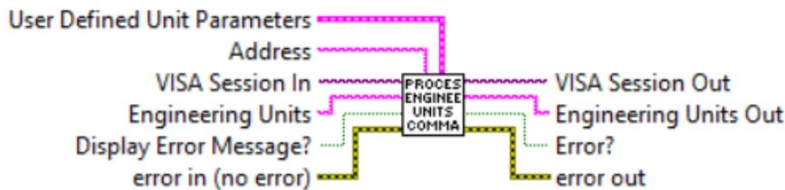
Sets/Reads currently selected mass flow units of measure. When "Engineering Units" terminal is empty this Sub-VI performs "Read" function. "User Defined Unit Parameters" cluster only required to set "USER" mass flow units. See XFM user manual Paragraph 8.3 for the list of supported mass flow units of measure.
