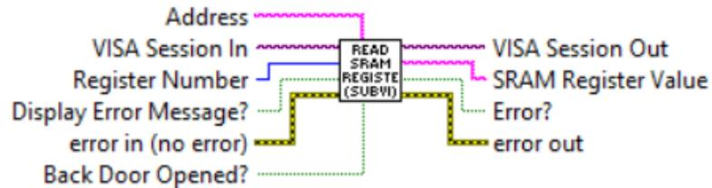
Reads instruments SRAM registers. Use this Sub-VI for diagnostic purposes. If "*Back Door Opened?*" terminal is set to "False" this Sub-VI performs "Open Back Door" commands first and then read requested SRAM register. To improve response time user may issue "Open Back Door" command in advance and then set "*Back Door Opened?*" terminal value to "True". Valid numbers for SRAM diagnostic registers are:
