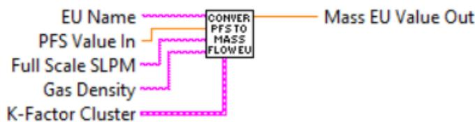
Converts mass flow PFS @ Factory STD conditions ([0.0-100.0%] notation) to the engineering units (STP conditions) which are wired to the "EU Name" terminal. This VI has to be run in the beginning of the instrument initialization and each time the instrument selected gas table or mass flow EU are changed.
