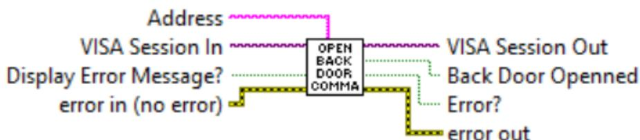
Opens Back Door for accessing instrument's diagnostic volatile memory (SRAM) registers.
