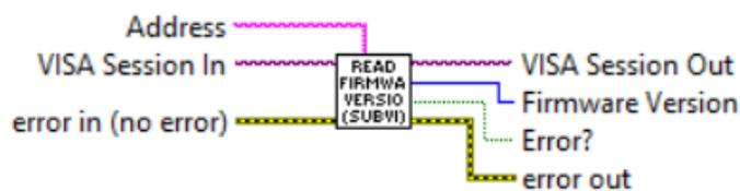
Reads instrument's firmware version and returns unsigned 32 bits integer which represents last to digits of the firmware revision (e.g. 9 for device with firmware version of 1.09). The firmware revision can be used to determine if instrument supports additional ASCII commands which were added to Ver. 1.10 of the XFM firmware.
