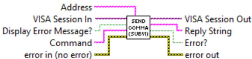
Sends the specified ASCII command to the instrument. Returns response as a string (unedited) which represent instrument's response for particular ASCII command (see Paragraph 8.3 in the XFM operating manual for the list of supported ASCII commands).
