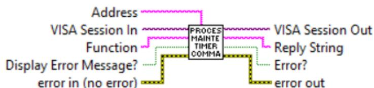
Reads/Resets instrument's maintenance timer. When "R" string is wired to the "Function" input terminal the instrument replies with floating point string representing current maintenance timer value in hours. When "C" string is wired to the "Function" input terminal the maintenance timer is set to zero and instrument replies with "CC" string.
