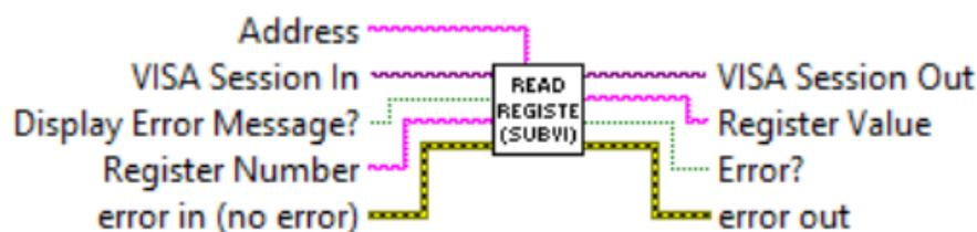
Reads single EEPROM register. Valid values for decimal string wired to the "Register Number" terminal are from 0 to 50 and from 100 to 134. Returns response as a string (unedited) which represent EEPROM register value.
