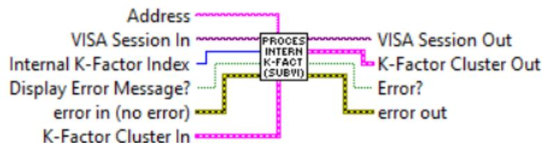
Applies Internal K-Factor to currently selected Gas Table. If successful returns "*K-Factor Index*", "*Gas Name*" and floating point number with "*K-Factor Value*" in the K-Factor cluster. K-Factor does not work with %FS engineering unit. Valid Internal K-Factor Indexes are from 0 to 35. To apply currently selected Internal K-Factor Index set "*Internal K-Factor Index*" terminal value to -1.
