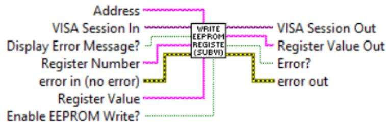
Writes specified value to the to the instruments corresponding EEPROM register . Returns response as a string (unedited) which represent EEPROM register value.
