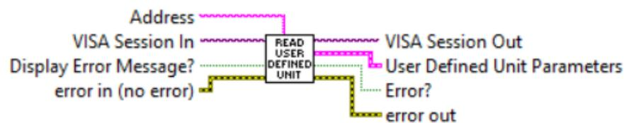
Reads current User Defined Unit parameters. If successful returns "User Defined Unit Parameters" cluster of strings containing floating point "Conversion Factor" to l/min value, "Time Base" string [M, H, S] and "Use Density" string [Y, N].
