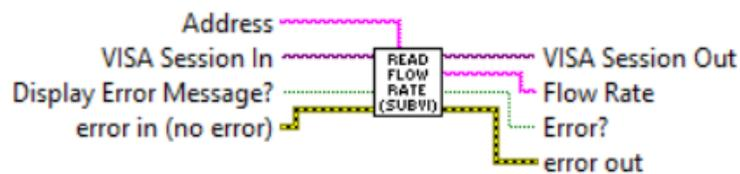
Reads the instrument's Mass flow reading value (floating point string) in currently selected mass flow units of measure.
