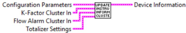
Takes key instrument configuration parameters from device "*Configuration Parameters*" "*K-Factor*", "*Flow Alarm*" and "*Totalizer*" clusters and combines them in to the "*Device Information*" cluster. This sub-VI can be run at the beginning of a program outside the main loop and should be re-run every time the instrument address is changed (for RS-485 interface).
