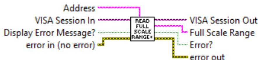
Reads instrument full scale range in SLPM. The full scale range value always based on selected gas table.
