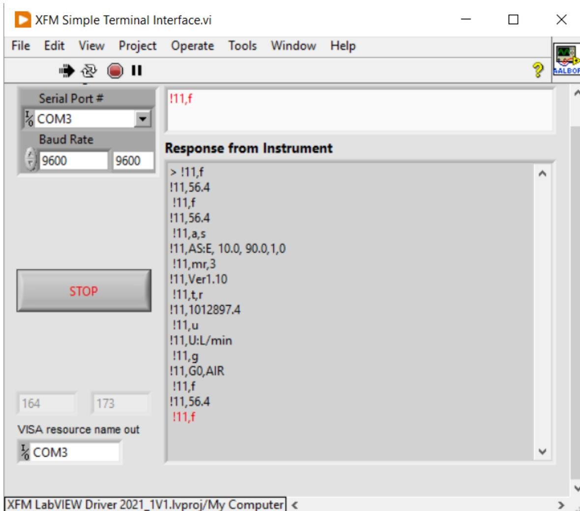
Example VI for communicating with AALBORG XFM instruments via serial communication interface using ASCII commands set (see XFM instrument operating manual for complete list of supported commands). For RS485 interface the start character is always ! and two characters of address with coma delimiter in the end must be submitted before each command (see example below).
