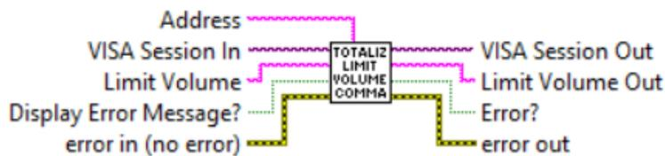
Sets Totalizer "*Limit Volume*" parameter. Wire floating point string to "*Limit Volume*" input terminal to set desired Totalizer "*Limit Volume*" parameter. The Totalizer "*Limit Volume*" value must be in currently selected (not time based) units of measure. Refer to XFM ASCII commands set (Paragraph 8.3 in the XFM operating manual) to determine valid values for "*Limit Volume*" input terminal.
