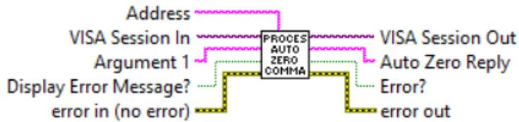
Performs Auto Zero function for the XFM instruments. Refer to XFM ASCII commands set (Paragraph 8.3 in the XFM operating manual) to determine valid values for "Argument 1" input terminal.
