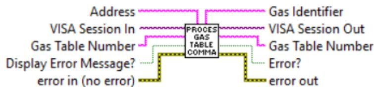
Sets/Reads currently selected Gas Table Number. When "*Gas Table Number*" terminal is empty this Sub-VI performs "Read" function. Valid values for "*Gas Table Number*" parameter are decimal strings from 0 to 9.
