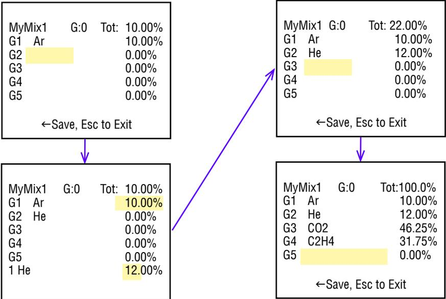
**Figure 27:** Mixture with 4 Components Ready to be Saved
