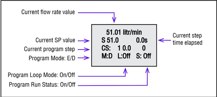
Figure 36: Instrument PI Screen #7 with PSP parameters
