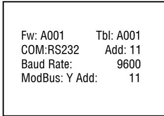
**Figure 7:** DPC Firmware and Communication Interface Information Screen
