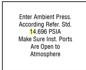
**Figure 41:** Entering Ambient Pressure from Reference Standard
