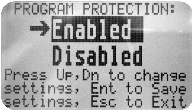
Pressing the **UP** or **DN** button to select the Disabled option and then the **ENT** button to save settings will disable program protection.
