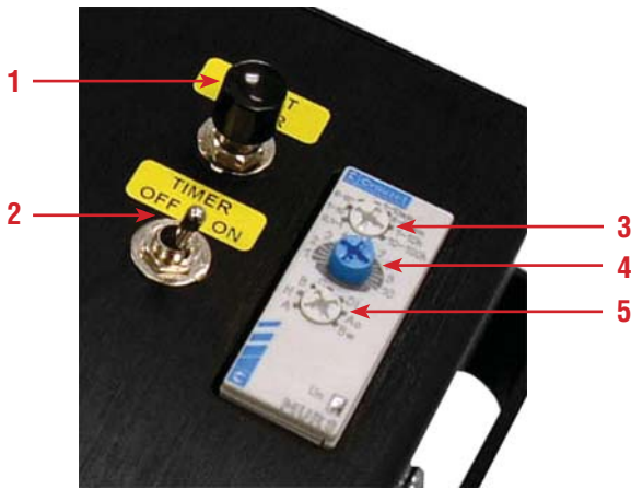
FIGURE 7: LOCATION OF MUR 3 TIMER CONTROLS
