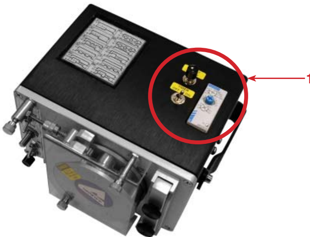
FIGURE 6: LOCATION OF MUR 3 TIMER CONTROLS
